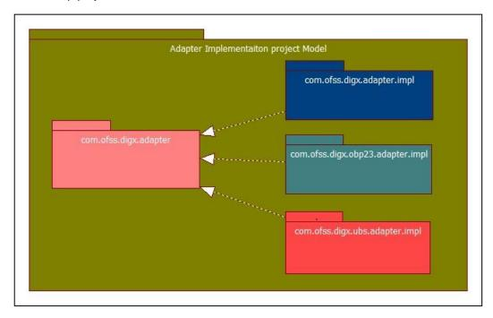
In above model, project **com.ofss.digx.adapter** contains all the adapter specifications (Java Interface). The concrete implementation classes of the adapter interfaces will reside in the host specific adapter implementation project.
